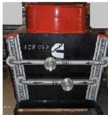
Remote radiator for Secondary circuit
